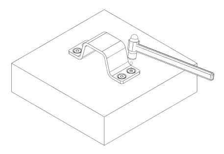
7. Use a hammer to hammer in the steel balls. This will ensure that the Ground Anchor is fitted securely.
