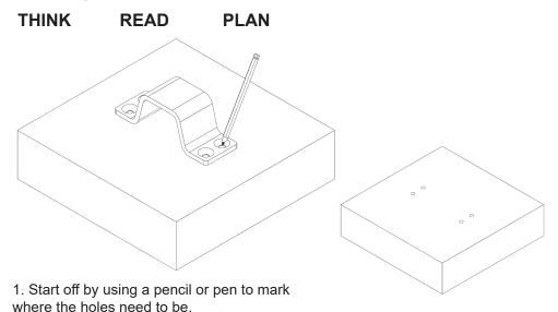
The ground anchor should be mounted on concrete or stone, and not on wood, porous stone, plaster wall, sand etc.
