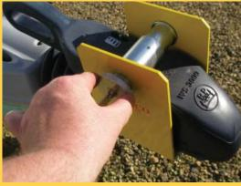
Push the 2 sections of the lockhole on the right hand side at ing bolt together and turn the
