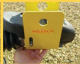
Position the hitchlock body underneath so that the stabiliser bolt is inserted in to the slot on the side
