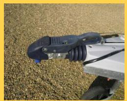
the push handle down into the bolt on the hitchlock engaged position
